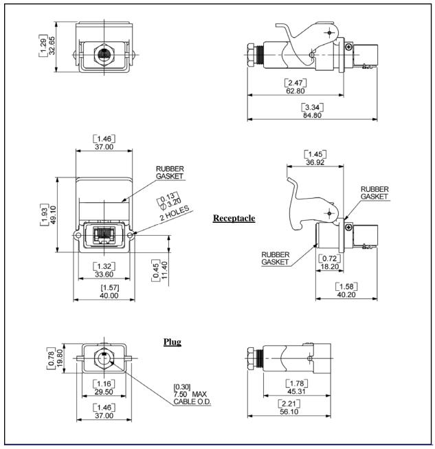
Receptacle termination can be an RJ, USB or discrete wires.
